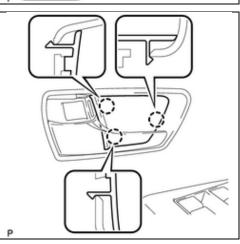
a. Engage the 3 claws and install the front door inside handle bezel plug.
