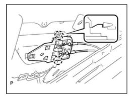
e. Disengage the 2 claws and disconnect the front door inside handle sub-assembly.
