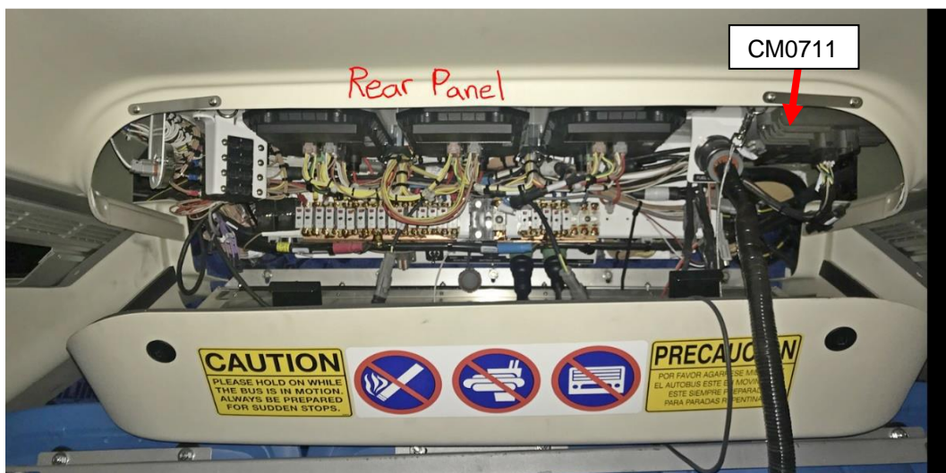
Figure 5: Rear panel and CM0711 module location
