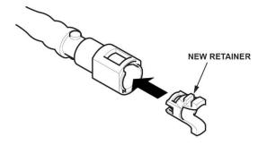
41. Connect the fuel line quick-connect fitting.
