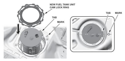
38. Turn the fuel tank unit cam lock ring by hand, and slide the fuel tank unit cam lock tabs to the positioning edge as shown.
