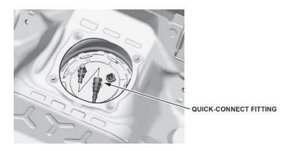
42. Connect the fuel tank unit connector.
