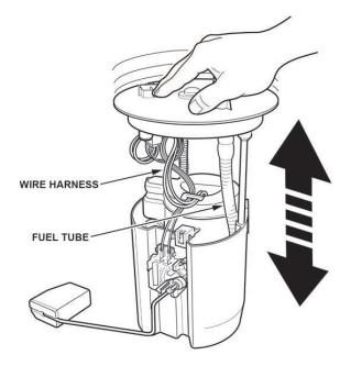
36. Install the fuel tank unit into the fuel tank with a new O-ring.
