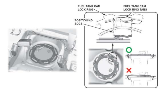
36. Turn the fuel tank unit cam lock ring by hand, and slide the fuel tank unit cam lock tabs to the positioning edge as shown.
