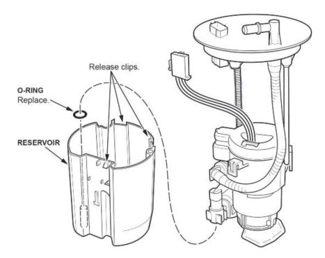
24. Release the three clips at the base of the fuel pump assembly and remove it from the fuel filter.
