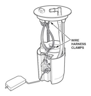
20. Press the tab on the fuel level sensor to release the lock. Then, push up on the fuel level sensor.
