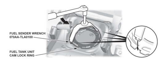
Turn the fuel tank unit cam lock ring counterclockwise to unlock it. NOTE: Make sure to keep the fuel sender wrench from floating.
