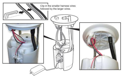
32. While compressing the fuel tank unit, make sure the movement is smooth and the fuel tube and wiring harness do not stretch, pinch, or bind.
