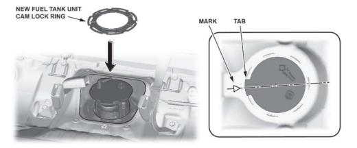
35. Tighten the fuel tank unit cam lock ring.
