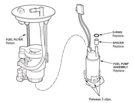
25. Pull the fuel pump assembly out of the fuel filter.
