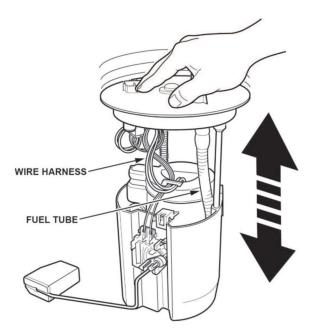
33. Install the fuel tank unit into the fuel tank with a new O-ring.
