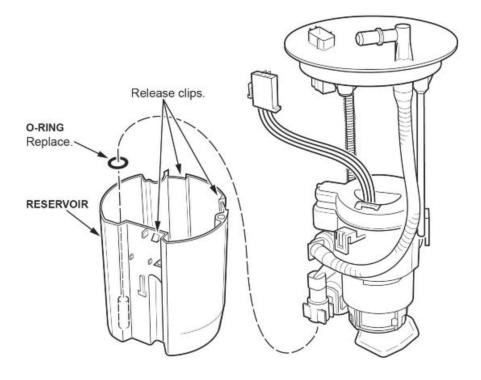
23. Remove the fuel filter assembly from the reservoir by releasing the three clips.
