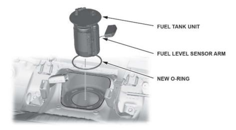
34. Line up the tab of the fuel tank unit as shown, and partially install the new fuel tank unit cam lock ring.
