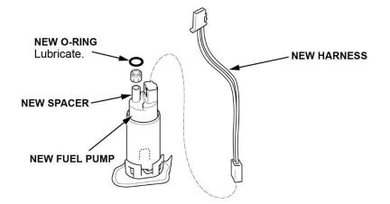
30. Place the fuel pump on a bench, then install the filter to the fuel pump.
