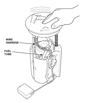
36. Insert the fuel tank unit partially into the fuel tank with a new O-ring.
