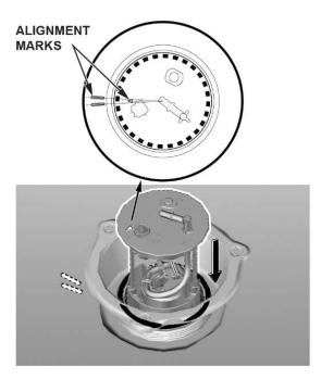
38. Align the mark on the new locknut to the start of the thread on the fuel tank.
