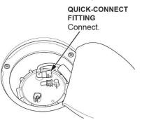
44. Connect the fuel tank unit connector.
