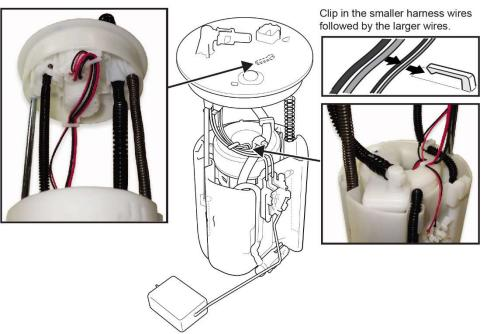
35. While compressing the fuel tank unit, make sure the movement is smooth and the fuel tube and wiring harness do not stretch, pinch, or bind.
