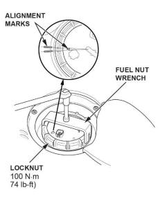
41. If the marks do not line up, friction between the fuel tank unit and the locknut may cause the fuel tank unit to turn while tightening. Observe the difference (shaded area), and loosen the locknut until the fuel tank unit can be rotated. Rotate the fuel tank unit **counter-clockwise** by the same amount, and repeat the tightening process.
