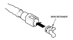
43. Connect the fuel line quick-connect fitting.
