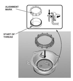
39. Press down on the fuel tank unit while turning the locknut clockwise by hand.
