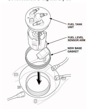
40. Line up the marks on the fuel tank and fuel tank unit as shown, then insert the fuel tank unit.
