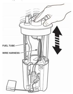
39. Partially insert the fuel tank unit into the fuel tank with a new base gasket.
