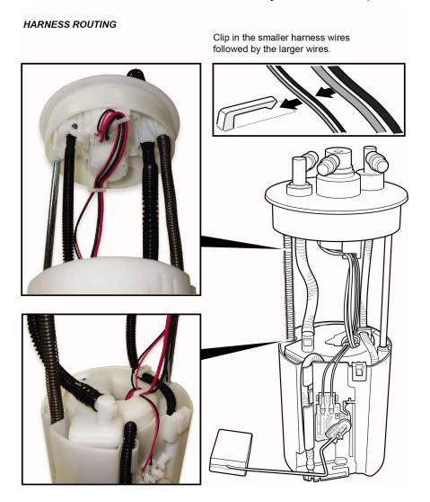
38. While compressing the fuel tank unit, make sure the movement is smooth and the fuel tube and wiring harness do not stretch, pinch, or bind.
