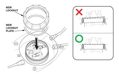
42. Tighten the fuel tank unit locknut to the specified torque using the fuel sender wrench.
