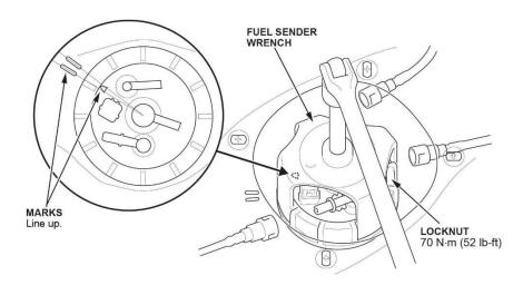
43. *If the marks do not line up*, friction between the fuel tank unit and the locknut may cause the fuel tank unit to turn while tightening. Observe the difference (shaded area), and loosen the locknut until the fuel tank unit can be rotated. Rotate the fuel tank unit **counter-clockwise** by the same amount, and repeat the tightening process.
