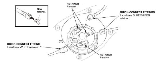
45. Connect the quick-connect fittings to the fuel tank unit.
