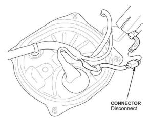
18. Remove the access panel from the floor.
