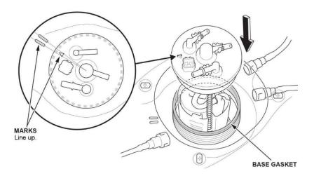
41. Hold the fuel tank unit vertically, and tighten the new fuel tank unit locknut with a new locknut plate by hand.
