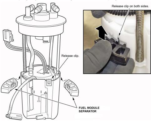
30. Release the three clips at the base of the fuel pump assembly.
