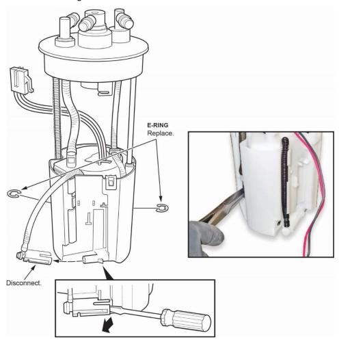
28. Disconnect the joint at the bottom of the reservoir.
