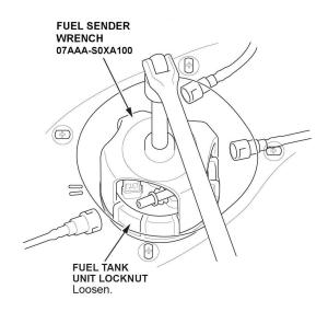
22. Remove the fuel tank unit locknut, then remove the fuel tank unit.
