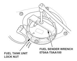
12. Remove the fuel tank unit.
