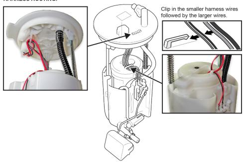
32. While compressing the fuel tank unit, make sure the movement is smooth and the fuel tube and wiring harness do not stretch, pinch, or bind.
