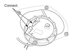
40. Connect the fuel tank unit connector.
