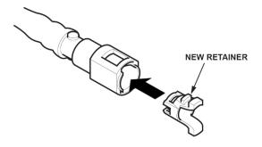
39. Connect the fuel line quick-connect fitting.
