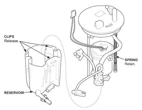
22. Release the three clips at the base of the fuel pump assembly and remove it from the fuel filter.
