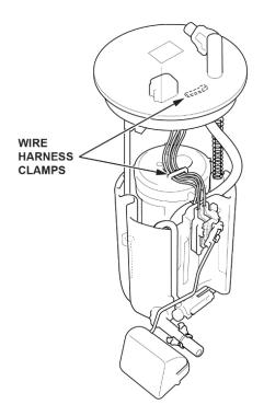
16. Press the tab on the fuel level sensor to release the lock. Then, push up on the fuel level sensor.
