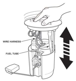
35. Install the fuel tank unit into the fuel tank with a new O-ring.
