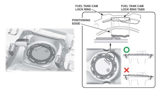
38. Turn the fuel tank unit cam lock ring by hand, and slide the fuel tank unit cam lock tabs to the positioning edge as shown.
