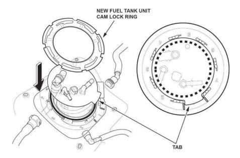
56. Connect the fuel vent tube and fuel tank vapor recirculation tube by slightly turning the fuel tank unit counterclockwise.
