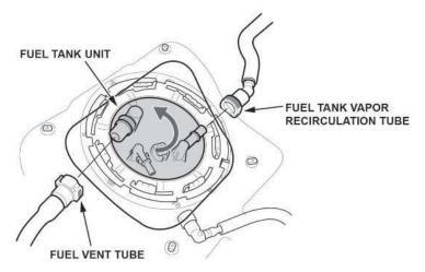
57. Turn the fuel tank unit cam lock ring by hand, and slide the fuel tank unit cam lock tabs to the positioning edge as shown.
