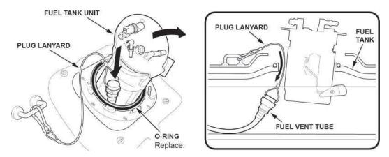
34. Remove the fuel tank unit with the O-ring.
