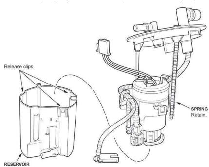
42. Release the three clips at the base of the fuel pump assembly and remove it from the fuel filter.
