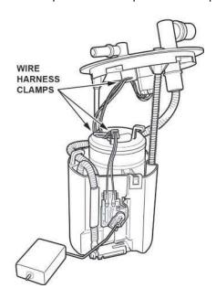
37. Press the tab on the fuel level sensor to release the lock. Then, push up on the fuel level sensor.
