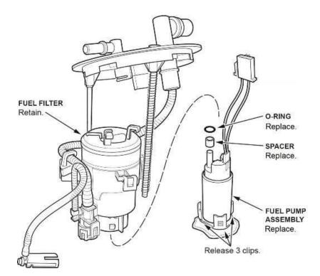
43. Install the new spacer, O-ring, and wire harness to the new fuel pump.
