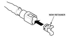
60. Connect the fuel line quick-connect fitting and connector.
