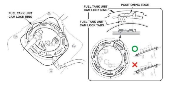
58. Tighten the fuel tank unit cam lock ring by turning clockwise using the fuel sender wrench.
