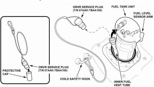
54. Remove the ORVR service plug from the child safety seat hook, and install the provided protective cap.
