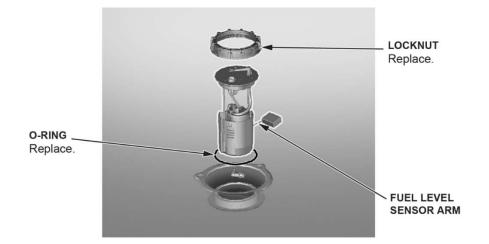
21. Prepare the fuel tank unit and parts to be replaced.
