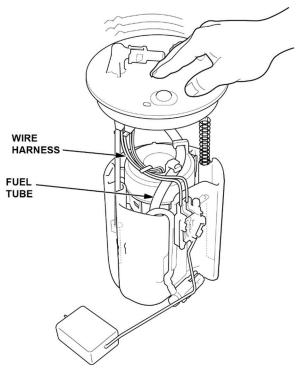
36. Insert the fuel tank unit partially into the fuel tank with a new O-ring.
