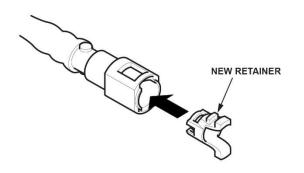
42. Connect the fuel line quick-connect fitting.
