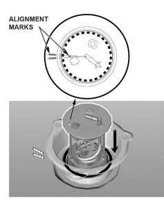
38. Line up the mark on the new locknut to the start of the thread on the fuel tank.
