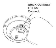
43. Connect the fuel tank unit connector.
