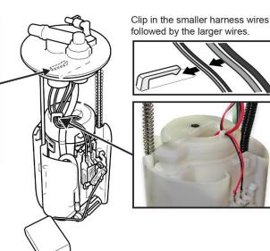
33. While compressing the fuel tank unit, make sure the movement is smooth and the fuel tube and wiring harness do not stretch, pinch, or bind.
