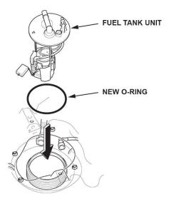
35. Line up the mark on the fuel tank unit to the marks on the fuel tank, then insert the fuel tank unit into the fuel tank. NOTE: To avoid any leaks, check the O-ring, either visually or by hand, to make sure it is not pinched.
