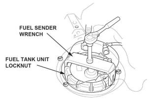
15. Remove the fuel tank unit.
