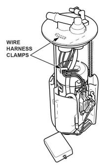
18. Press the tab on the fuel level sensor to release the lock. Then, push up on the fuel level sensor.
