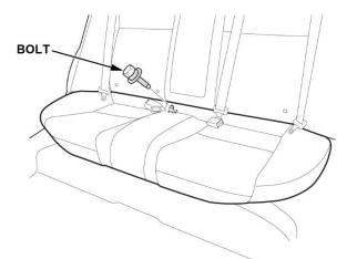
5. While pushing down on the rear seat cushion, pull the seat hook handles to release the hooks.
