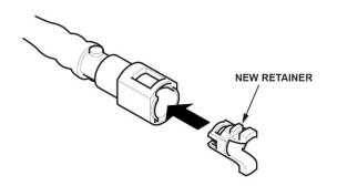
40. Connect the fuel line quick-connect fitting.
