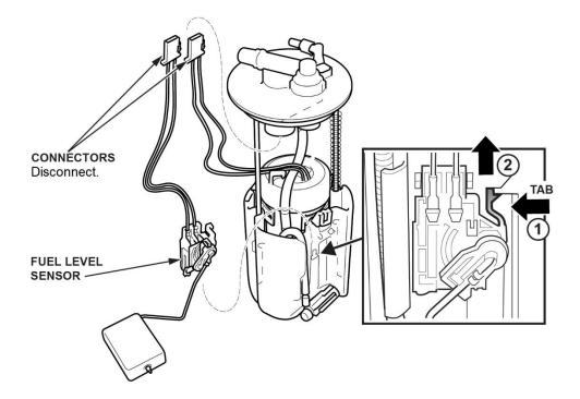
19. Disconnect the fuel level sensor harness and remove the fuel level sensor from the fuel tank unit.
