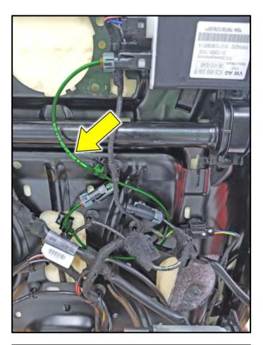
If present, disconnect and discard 69Z4 PODS repair wiring harness <arrow>.
