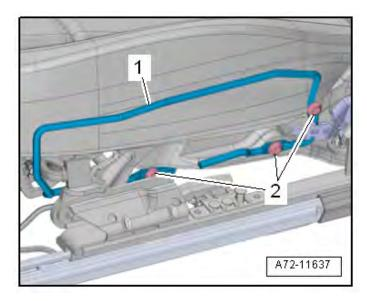
Remove the bolts <2> and remove the bracket <1>.
