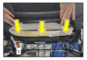
Ensure seat foam <arrows> is fully engaged over the rear of the seat pan <1>.
