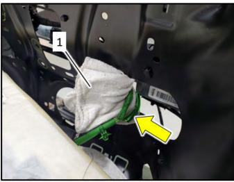
Place a protective cloth <1> between the seat pan openings and wiring harness <arrow> to prevent damage to the seat wiring harness.
