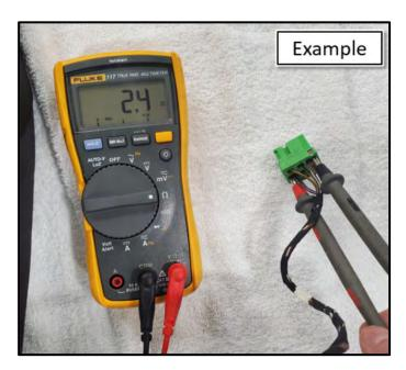
Before removing the sensor mat from the seat cushion, verify the resistance of the seat heater element (if equipped):
