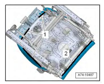
• Engage the molding <1> and <2> onto the seat pan.
