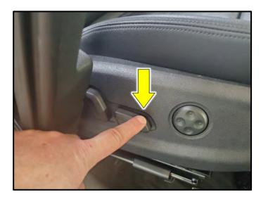
• Press down on the seat bottom tilt adjustment.
