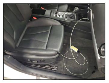
Route the 12V power cable so that it does not rest on the passenger seat.
