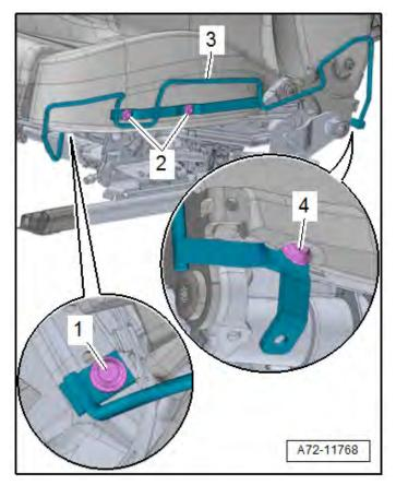
Remove the bolts <1, 2, and 4> and remove the bracket <3>.
