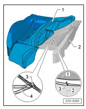
• Remove cover <1> from the cushion <2> and cut upholstery clips <3> using pliers <4>.
