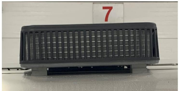
**Step Two:** Replacing the bolts that hold the A/C to the roof. You will be replacing the bolts one at a time by removing one bolt and then putting in the new bolt, Then torquing it to 40 inch pounds before taking out the next one.
