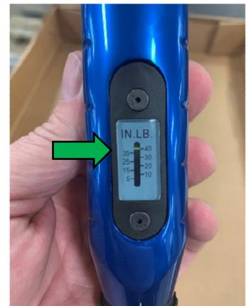
**Notice:** If any of the four bolts are stripped out and will not tighten to 40 Inch pounds the A/C will need to be replaced and you will need to use the new bolts and foam on the new A/C unit.
