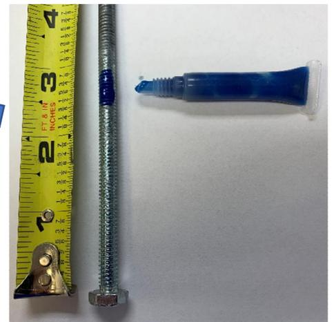
2. Put some lock tight on the grade 5 bolt about 2 1/2 inches to 3 inches up from the head of the bolt.
