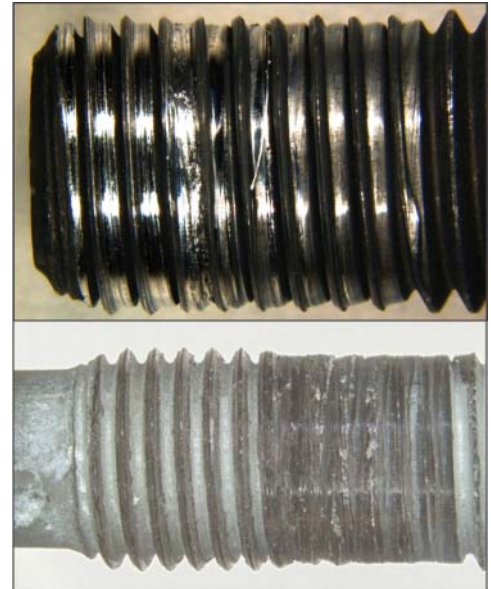
Damaged thread on actuator
