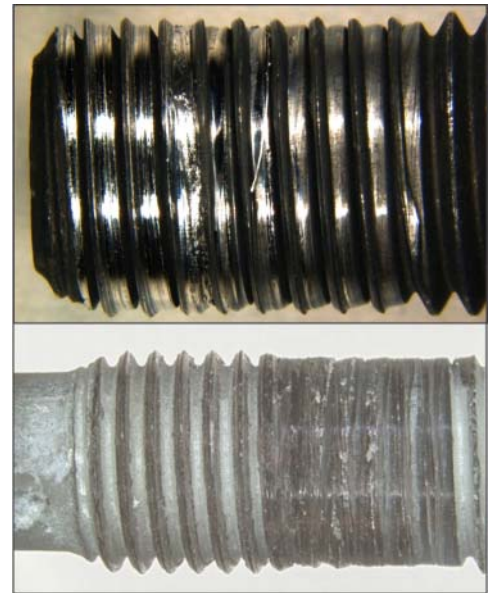
Damaged thread on actuator
