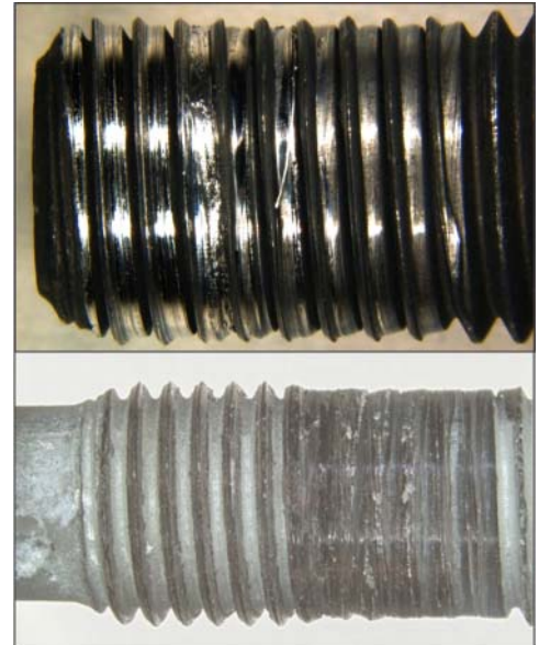
Damaged thread on actuator
