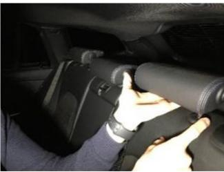
If the headrest cannot be lifted out of the seat, the positive stop is present. This headrest is thereby OK.
