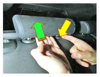
1. On either outer headrest, squeeze the headrest height release button (yellow arrow) at the seatback top retaining collar.
