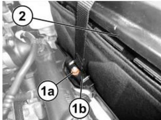
**Figure 4 – Battery Retaining Belt**
