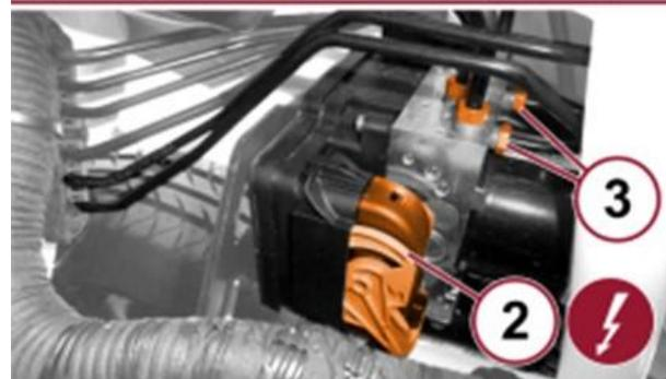
**Figure 10 – ABS Electrical Connectors**
