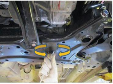
On Hole C and Hole D, insert nozzle until the nozzle is over weld nut. Make surethe anti-corrosion agent is not put on the inner surface of weld nut. Should anti-corrosion agent get on the inner surface of the weld nut; please remove by using Universal Absorbent Pads.
