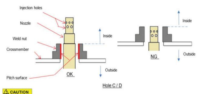
On Hole C and Hole D, insert nozzle until the nozzle is over weld nut. Make sure the anti-corrosion agent is not put on the inner surface of weld nut. Should anti-corrosion agent get on the inner surface of the weld nut; please remove by using a Universal Absorbent Pad.
