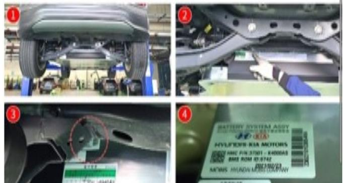
A-3. Use STUI camera photo upload function to save and submit photo to HMA of the BSA label.
