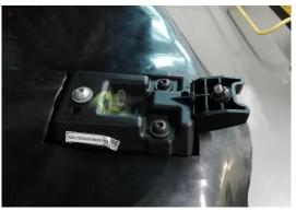
5. Perform the same procedure (from point 1 to point 4) for screws number 2 and number 3. remembering to replace them one at a time and paying attention to not exceed the tightening torque.
