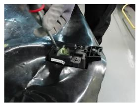
3. Hand tighten the new fixing screw provided in the kit (part number N91074202) and its washer (part number N10612001) completely.
