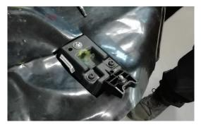
4. Tighten to torque using ONLY the torque wrench provided, code 61153001837 (or, as an alternative, code VAG 1783).
