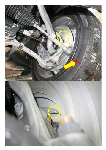
2. Carefully view into the front disc hub at the area circled.
