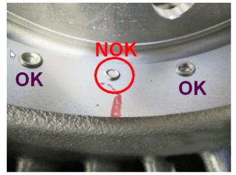
Determine if the rivet is correctly shaped per the 2 reference photos.
