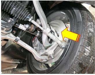
Inspect the left and right front brake disc rivet installation in the area of the arrow and if necessary, replacing the front brake discs.
