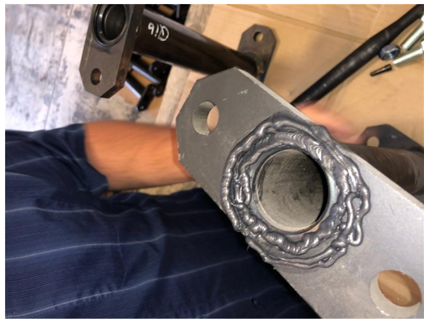
^ STEP 2: 1/8" BEAD AROUND HOLE (CALIPER SIDE)
