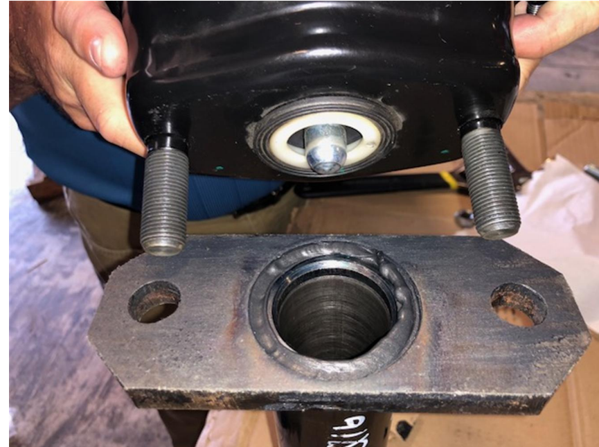
v STEP 1: 1/8" BEAD IN STEP (CHAMBER SIDE)
