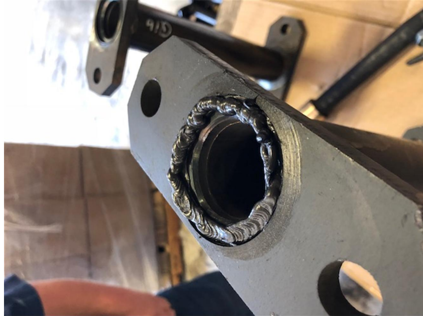
^ STEP 1: 1/4" BEAD IN STEP (CALIPER SIDE)
