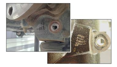
Inspect left front and right front wheel bearing housings and replace if necessary.
