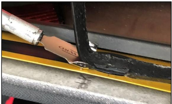
6. In the areas where the urethane did not adhere properly to the flange surface, the urethane will be easier to peel off as shown in the photo.
