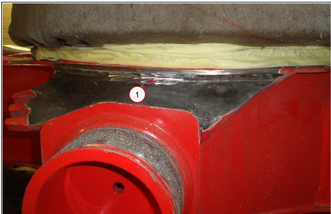
Illustration 09-53- 5: Area after grinding
