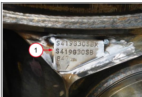
Illustration 09-53- 3: Remove part plate
