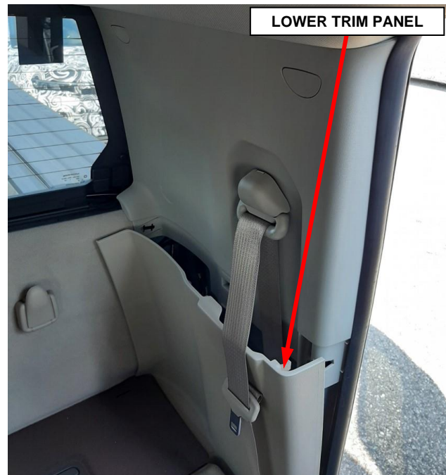
Figure 73 – C-Pillar Lower Trim Panel
