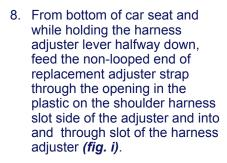
**Note:** Moving the harness adjuster lever up and down slightly can help feed the strap through the harness adjuster.
