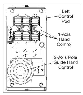
Figure 1 – Pole Guide Control Location
