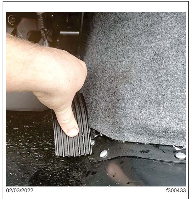
Fig. 8, Throttle Pedal with Insufficient Clearance
