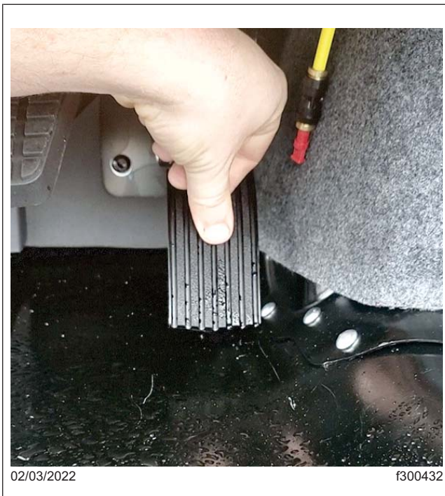
Fig. 1, Throttle Pedal with Sufficient Clearance
