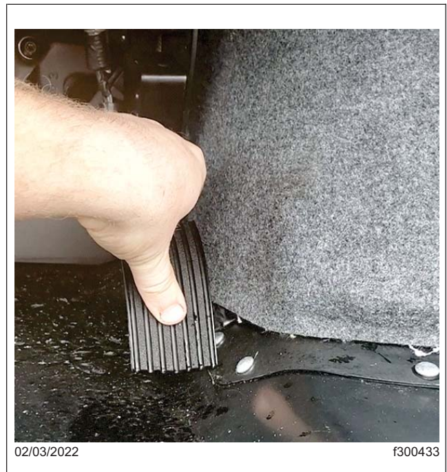
Fig. 2, Throttle Pedal with Insufficient Clearance
