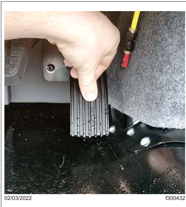
Fig. 7, Throttle Pedal with Sufficient Clearance
