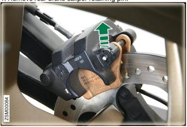
2. Remove rear brake caliper pin bolt. Tool: T25.
