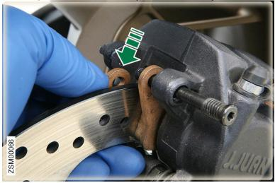
4. Remove both rear caliper brake pads.
