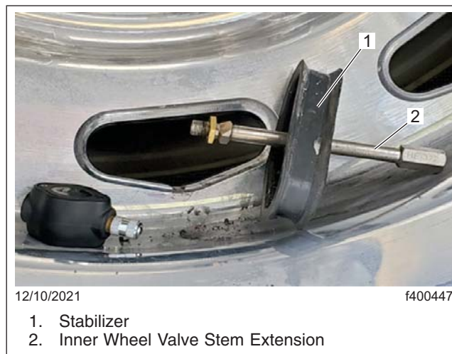
Fig. 1, Inner Wheel Valve Stem Extension and Stabilizer
