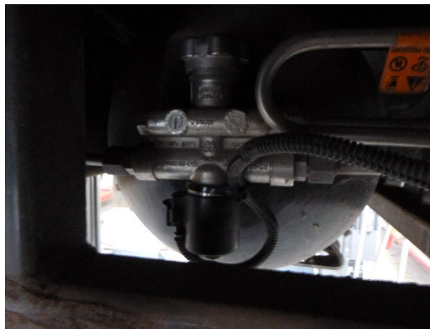
Fig. 7, When Securing the Harness and Connector, Allow for Strain Relief
