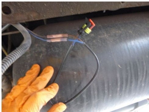
Fig. 5, New Connector Shown With Blue and Brown Wires
