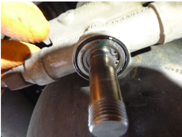
Fig. 8, Solenoid Removed Mount Location
