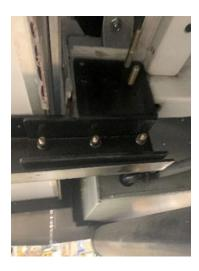
10. Reinstall the hydraulic leveling jacks in tandem with Step 11. <u>IMPORTANT NOTE</u>: Units equipped with Bigfoot leveling system will need to ensure the hydraulic foot and ram are reinstalled as a "washer" on the inside of the frame rail.
