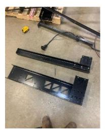
12. Install new cross member using 4 grad 8 hex bolts per side. Tighten bolts to 85 ft. lbs.
