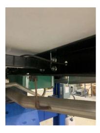
7. Remove all hydraulic jack hardware and zip tie jacks up and out of the way.
