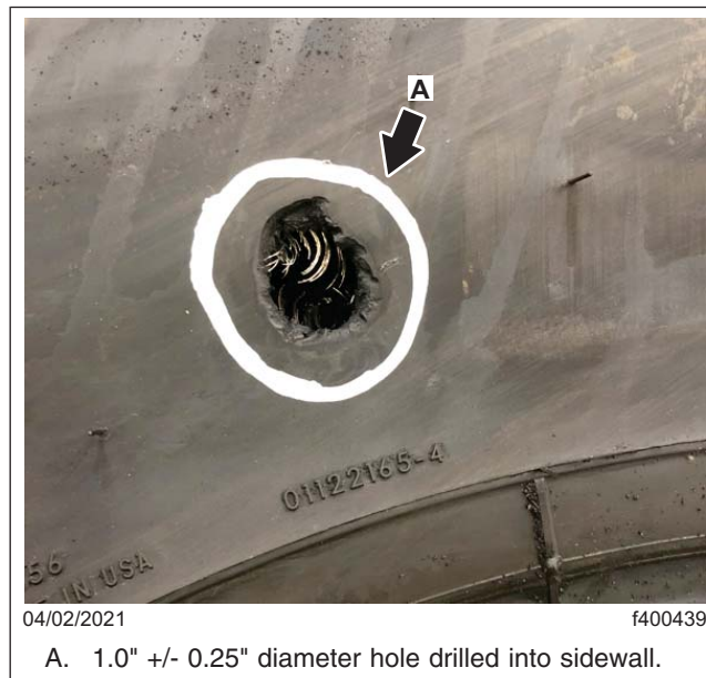
Fig. 9, Hole Drilled
