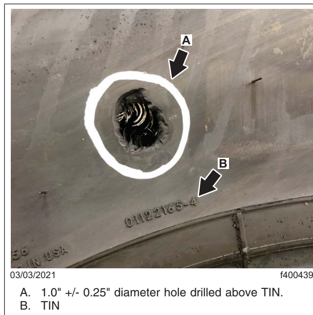
Fig. 7, Hole Drilled Above the TIN
