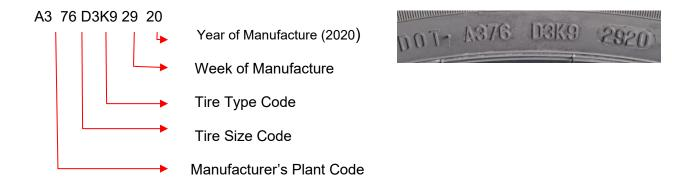
Tires made for use in the United States have a printed unique mold number located on both sidewalls of the tire.
