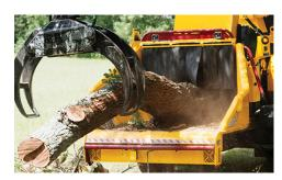
POWERFUL PERFORMANCE. Equipped with up to 11,674 lb (5295.2 kg) of pull-in force, this unit has optimized efficiency while working in tandem with the patented SmartFeed system to increase productivity when chipping large diameter logs.
