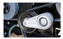
**AUTO BELT TENSIONERS.** Keeps proper belt tension at all times and extends belt life.
