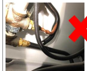
If the copper tubing is twisted or kinked it needs to be repaired or replaced. Only LPG qualified RV Technicians are approved to repair or replace copper tubing.
