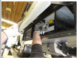
Before making any repairs make sure the propane tank solenoid (or tank valve on W24MB/FTB) is closed (OFF).
