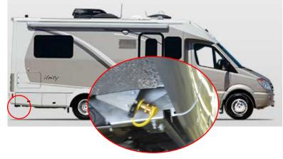
Use the BBQ hook up to burn off any propane still in the lines. The stove top can also be used, but may leave a small amount of propane in the lines.
