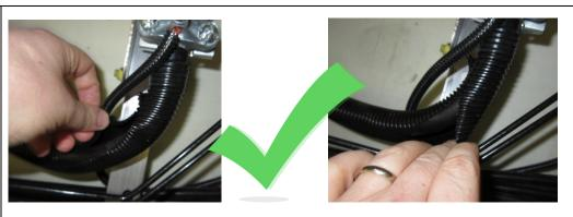
Wherever the propane hose makes a 90° corner, pull back the plastic tubing at the split
