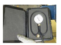
Connect a Manometer gauge to the BBQ hookup. Bleed down the system to 9 inches water column pressure to equalize the pressure on the input line and the output line of the regulator.
