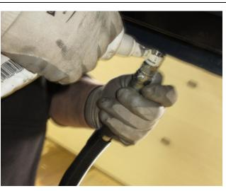
Apply Loctite 567 Thread Sealant (129-3251) to the threading of the hose
