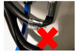
Wherever the propane hose bends, and kinks a repair will be considered necessary. Only LPG qualified RV Technicians are approved to repair or replace coper tubing.
