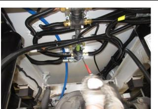
After it has been confirmed that the propane lines are leak free, reinstall all the hose and tubing clamps into the same holes that they were removed from.
