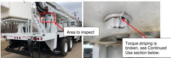
Figure 1. Area of unit to inspect rotation bearing bolts
