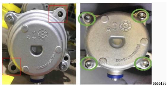
Note: The purpose of this service procedure is to inspect for the presence of missing bolts in the Transmission Auxiliary Fluid Accumulator Cover, an example of which is shown above.
