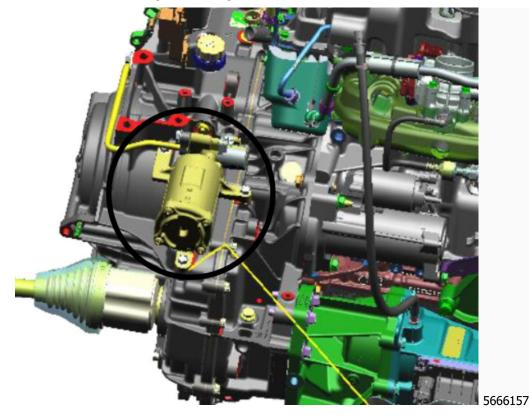
2. Looking straight up around the rear of the transmission, identify the transmission auxiliary fluid accumulator.
