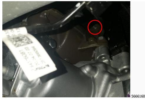
3. Visually verify the first bolt (circled above) is installed. You will be looking for the threads protruding from the transmission fluid accumulator housing for these vehicles to verify the bolt is installed.
