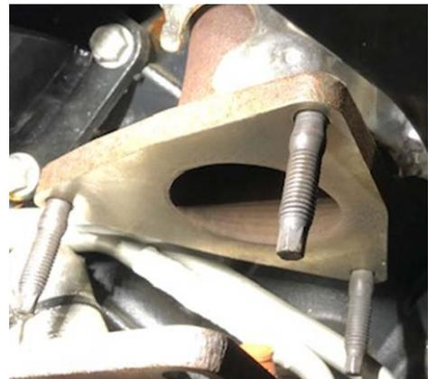
3. Tighten all of the exhaust studs fully into the exhaust manifold flanges.
