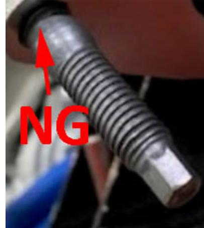
\*If any of the studs or nuts cannot be reused due to damage, replace them with OEM studs (ML296164) and nuts (ML296165).
