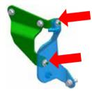
4. Connect the new vacuum exhaust hose through the shield and bracket before affixing it to the engine.
