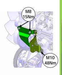
Clearance check on DMU=> 5mm
