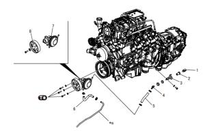
3. Reroute the vacuum exhaust hose and install the exhaust heat shields using the attached Modification Procedure.
