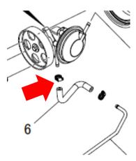
3. Assemble bracket and shield (M6, 5.2 ft.lbs.).
