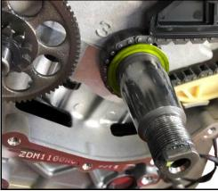
20. Fit the starter motor driven gear with the needle roller bearing cage on the **rotor assembly** (12) by rotating it slightly and applying a moderate force at the same time
