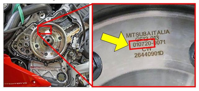
On the affected motorcycles, check the production date on the generator rotor (flywheel) and if one of the 6 production dates relating to potentially defective batches is found on the component, replacement will be necessary. The batches of generator rotors (flywheels) identified as potentially defective are: 280620, 290620, 300620, 010720, 020720, and 030720
