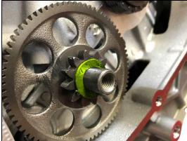
**22.** Install the rotor assembly on the crankshaft, ensuring that the starter motor driven gear engages with the idle gear
