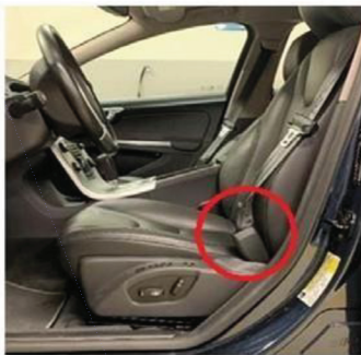
The seat belt lower fixing buckle rests in a position that is past the bolster of the seat
