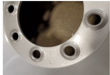
Properly Manufactured Wheel Correct Lug Nut Seat Identified by raised surface only around lug nut location
