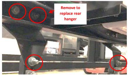
2. Install the flat hanger bracket at the rear of the exhaust as shown in the picture to the right.
