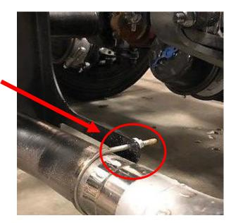
4. Using a center punch, mark the bottom rail 1" in from the edge of the rail and centered under the pump bracket.
