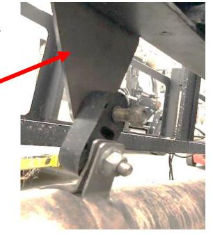
3. Loosen tail pipe U-bolt. Pull the exhaust pipe out approximately 3-4" so you can access the frame rail with a drill. Tighten the U-bolt enough to keep it out of the way during the drilling process.
