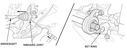
10. ILX Hybrid Only: Pry the inboard joint from the transmission using a pry bar. Remove the driveshaft as an assembly.
