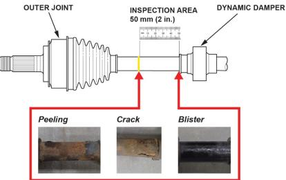
Is there peeling paint, cracks, or blisters on the driveshaft within 50 mm (2 in.) of the dynamic damper?
