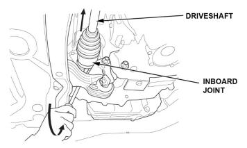
11. Insert the inboard end of the driveshaft into the differential until the set ring locks in the groove.
