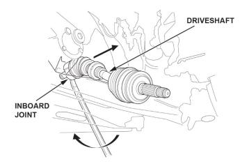
8. *ILX Only:* Drive the inboard joint off the intermediate shaft using a drift punch and a hammer. Remove the driveshaft as an assembly.
