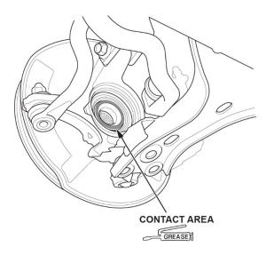
15. Install the outboard joint into the front wheel hub.
