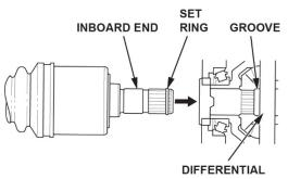
12. Left Driveshaft: Clean the areas where the driveshaft contacts the differential thoroughly with solvent. Dry the areas where the driveshaft contacts the differential thoroughly with compressed air.
